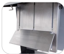
The articulating bag support supports the pouch during sealing then tilts down to dispense the pouch.
