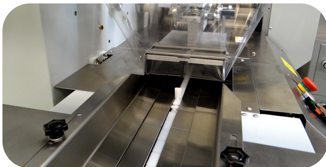
Delicate product conveyor with carrier card in-feed guide rails to handle product transitioning to the custom fixed former.
