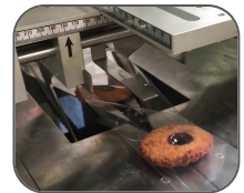
The Flow Wrapper 350T rapidly encloses the product in a tube of film before cutting and sealing the packages
